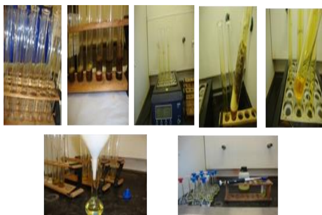
Fig. 1. Sample digestion ( aqua-regia )
