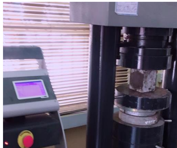
Figure 4. Compressive strength test
