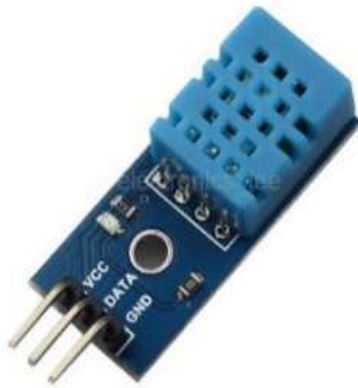
Figure 2. DHT11 Temperature and Humidity Sensor.
