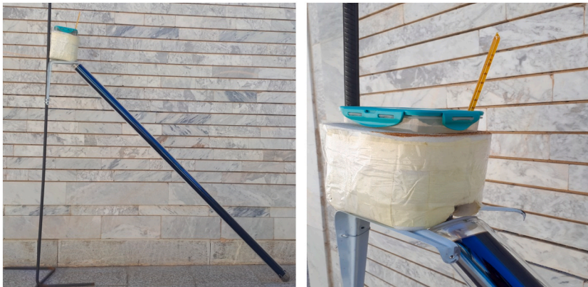
Fig. 4. The installation of a thermally insulated container above the HP tube.
