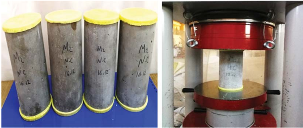
Fig. 1. Concrete Specimens before Crushing under Compression Machine
