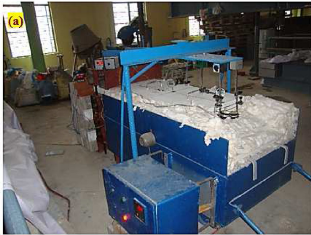
Fig. 2 – (a) Slab heating setup (b) Time – Temperature curve of furnace.
