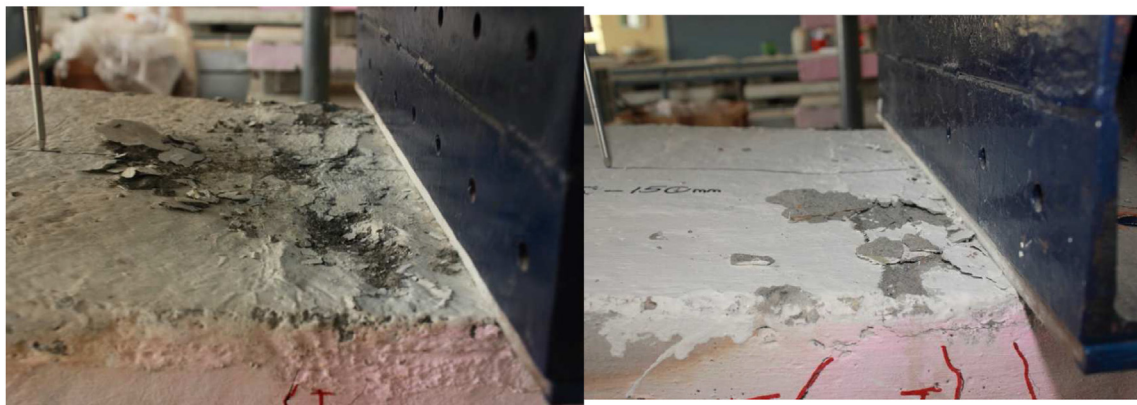
b) Initiation of Compression Failure in the Concrete Specimen under Mechanical Loading
