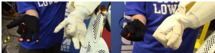
Figure (3): Shows the utilizing the Manus VR glove to control Valkyrie's hand
