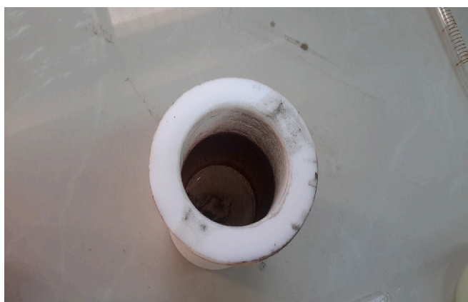
Fig. 2. The results of solvothermal synthesis of ZIF-8/Zeolite.
