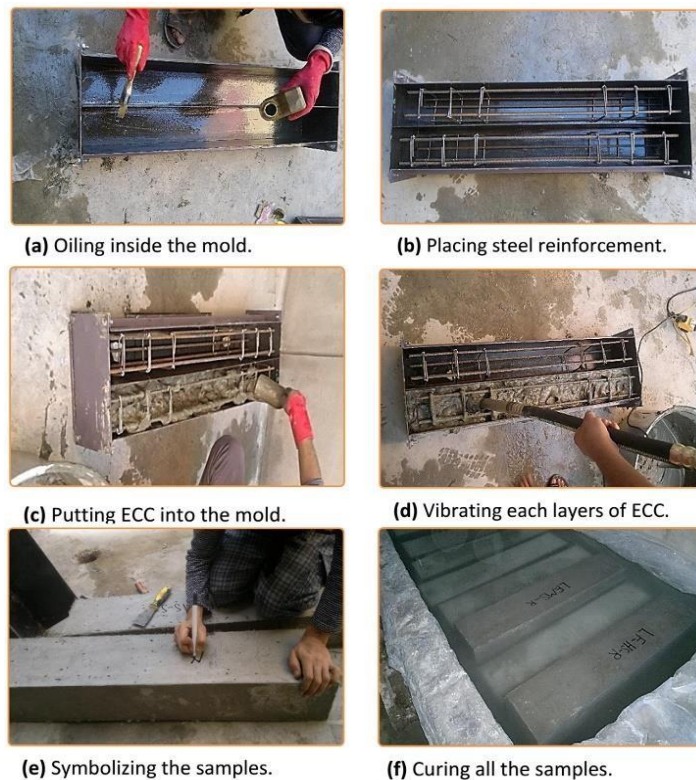
FIGURE 4. Casting and curing steps
