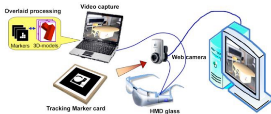
Figure 11. AR tracking & display process: the computer generated graphics are integrated into user's view.
