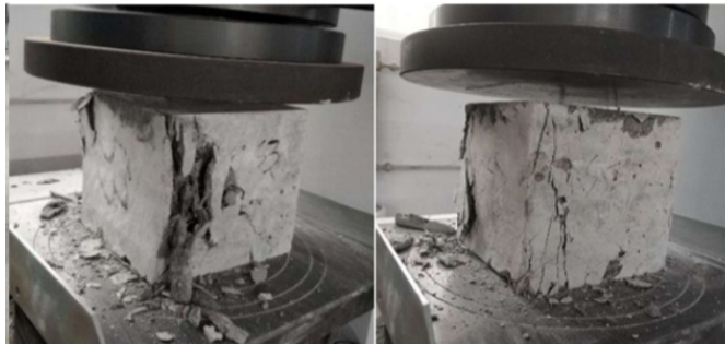
Figure(5) Specimen damage patterns after the cubic compressive strength test
