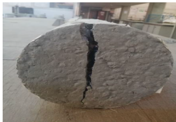
Figure(9) Damage patterns of specimens after cylinder tensile strength test
