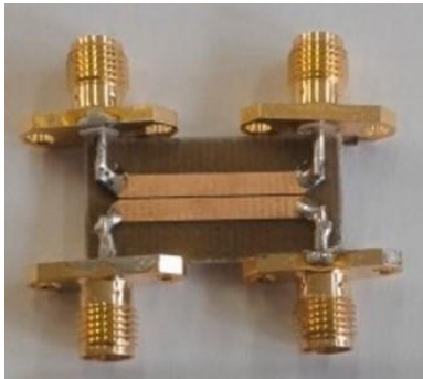
Fig. 8: Manufactured directional coupler
