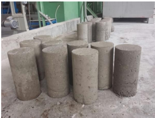
Fig-8 After Forms Removal
