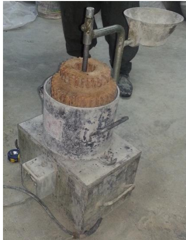
Fig -6 Modified Vebe apparatus.
