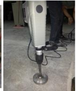
Fig.1- Cylindrical Molds (Φ15cm * 30cm) Fig.2- Modified Vibrating Hammer (+45 micron): 43.39%
