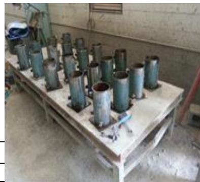
Fig.1- Cylindrical Molds (Φ15cm * 30cm) Fig.2- Modified Vibrating Hammer (+45 micron): 43.39%
