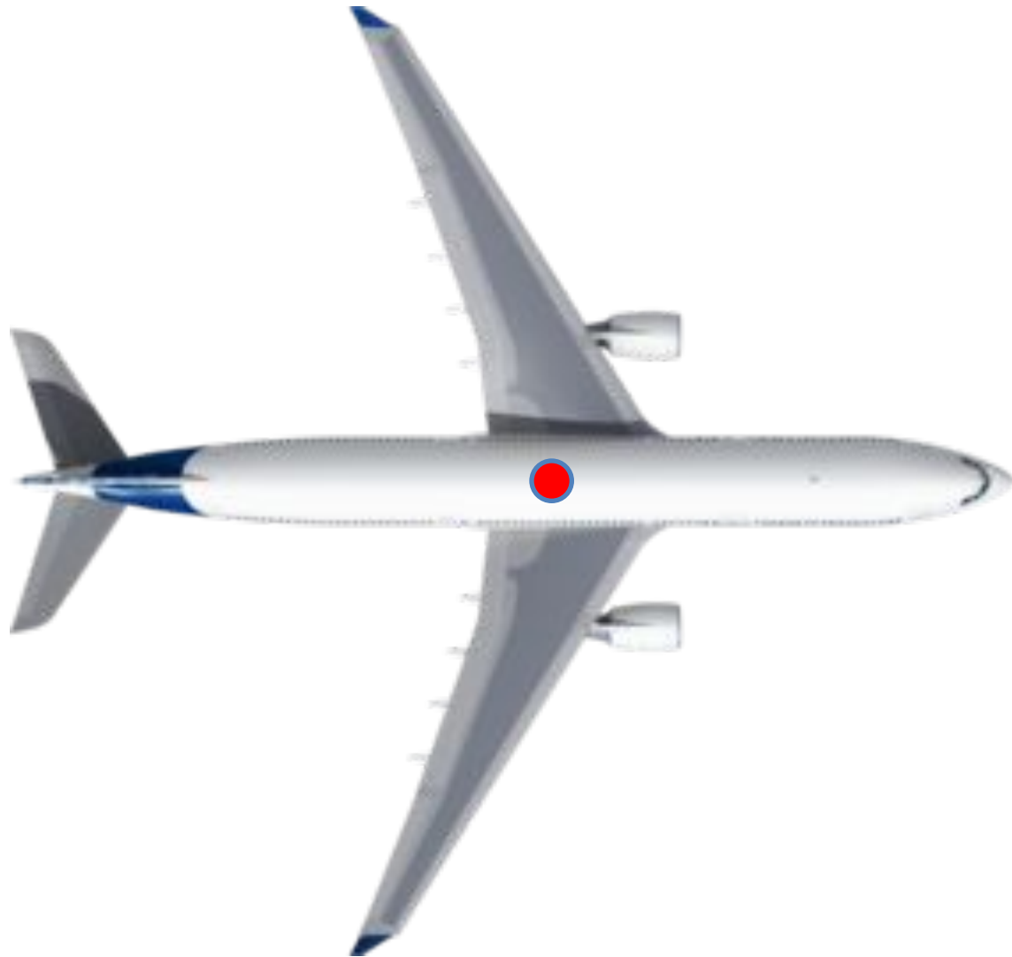
Figure 1: Main Beacon device position in centre mass of airplane
